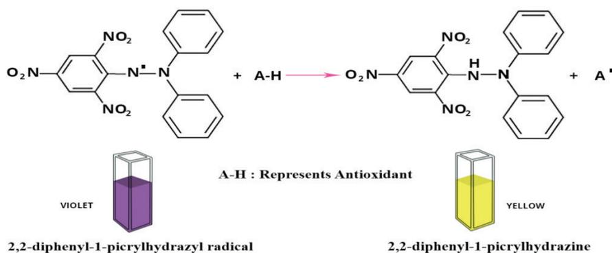
Fig. 1: Reduction effect of AH to DPPH.
