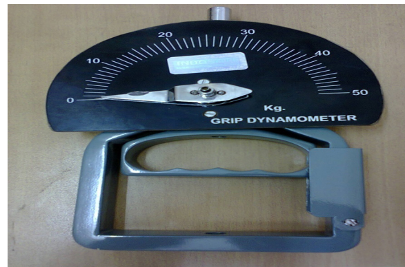
Figure 1 showing hand grip dynamometer to measure MVC
