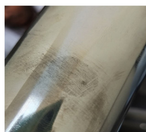
Figure 3: Development of latent fingerprint with the help of carbon powder on non- porous metal surface
