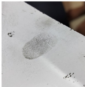
Figure 2: Development of latent fingerprint with the help of carbon powder on non- table.
