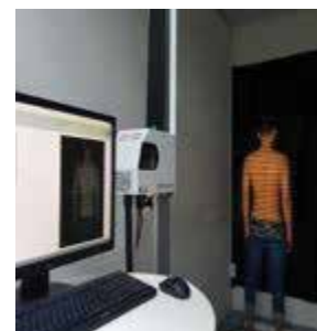
Figure 2: Measurement of the spine alignment using Formetric 4D
